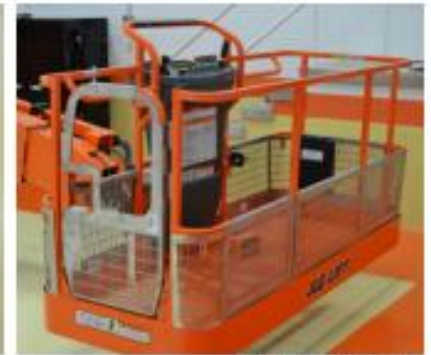
Mesh to Mid Rail
